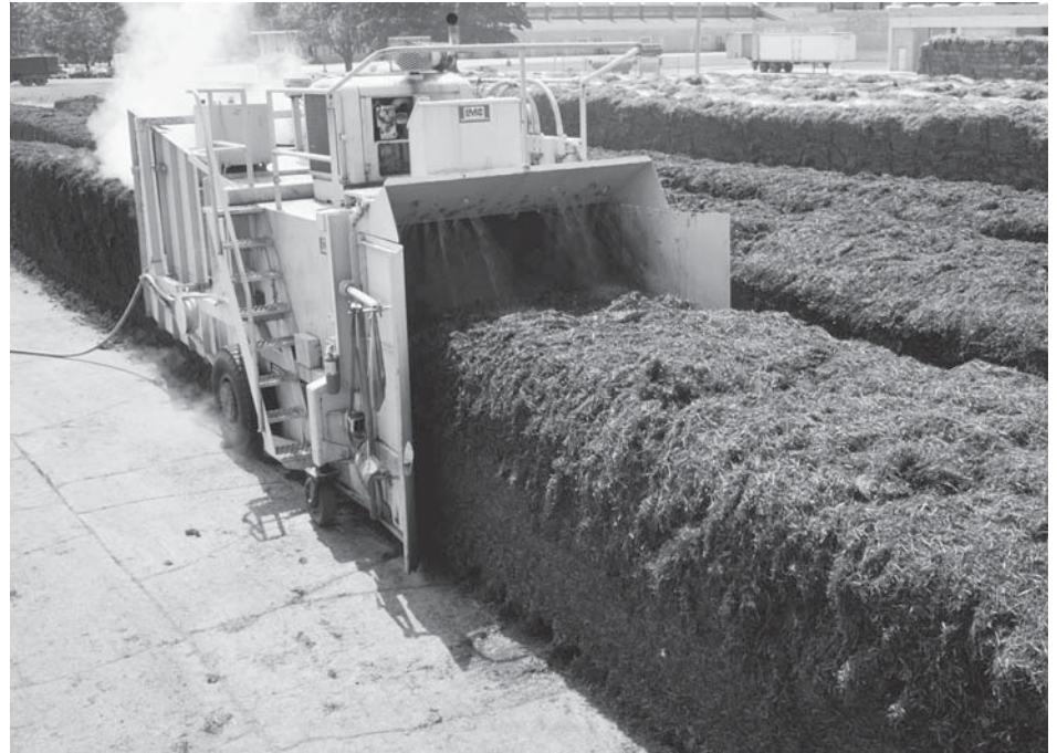
Figure 2. Self-propelled compost turner moving through a compost rick or pile.
